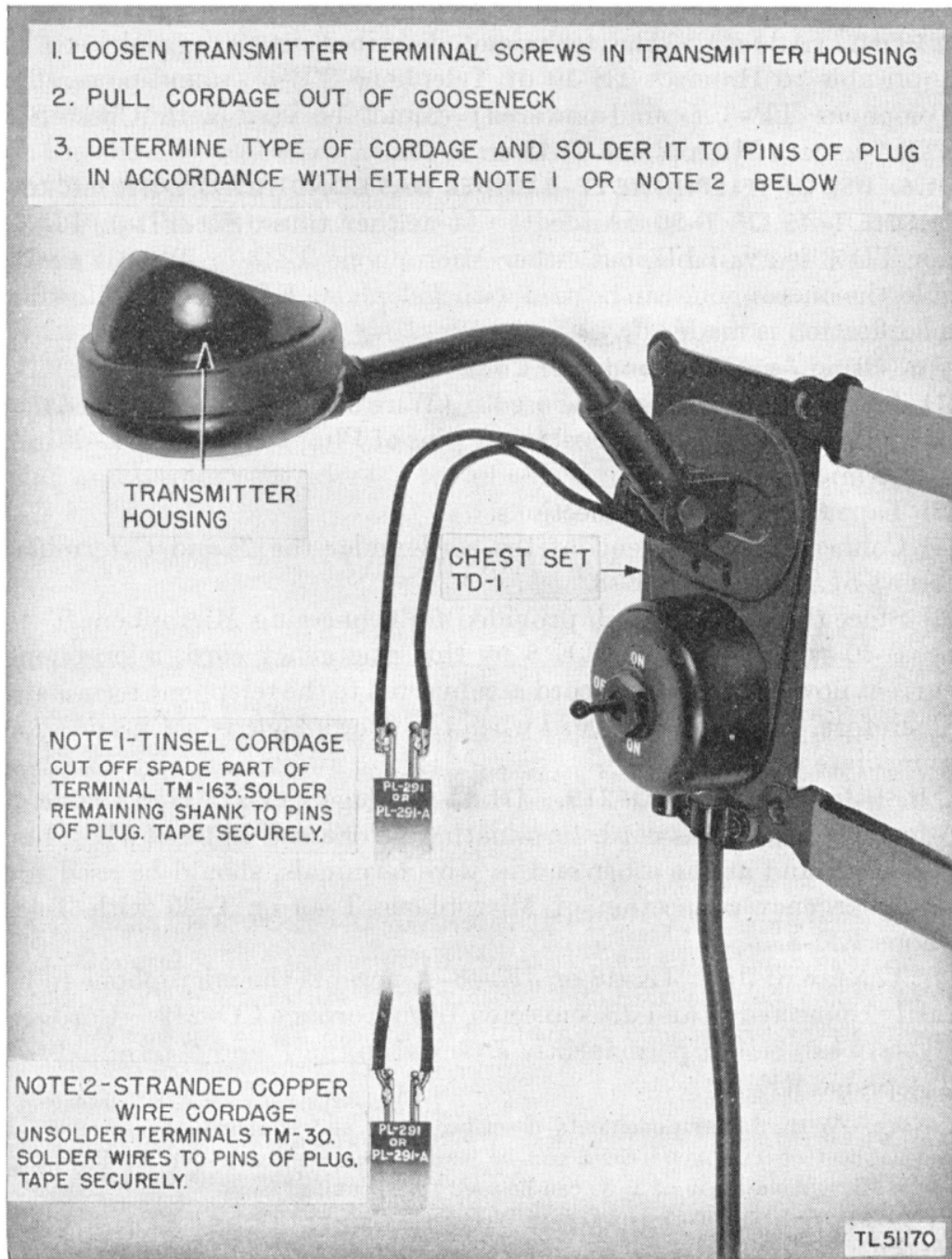
Figure 7.1.—Emergency use of Microphone T-45 or T-30 with Chest Set TD-1 or TD-2.
